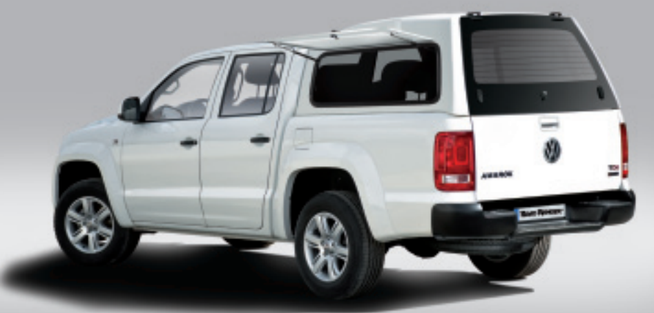
Hardtop BacPac Professional with lockable side access flaps (fiberglass, painted in hardtop colour) additionally equipped with carpet headlining Art. 6012 Art. 6015
