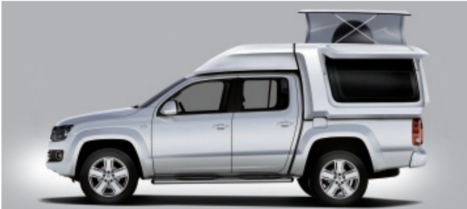
Vario-Top Professional with lifting roof and lockable side doors Art. 6042 (GPR painted in hardtop colour)
